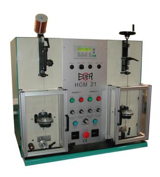
for sizing & polishing of the cylindrical die-bearings
