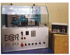
High Speed Grinding and Polishing Machines in semi-automatic version:
